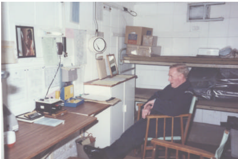
John Harding inside the ROC underground post at Daventry during the 1970s. Instruments evident on the wall are the Bomb Power Indicator, for measuring the intensity of the pressure wave from a nuclear explosion. On the desk are the training version of the Fixed Survey Meter, for measuring fallout radiation, and the BT Teletalk for communication with Control and other posts in the Cluster. The carrier receiver, over which an Attack Warning Red message would be received, is partially shown on the left hand edge of the photo. Food ration packs are on the double bunk bed in the background for use by the operational crew of 3 persons. Lighting was by a 12 volt battery powered 6 watt striplight, the battery being periodically charged by a petrol generating set. Ventilation of the post was achieved by opening and closing blastproof sliding vents that connected to a vent shaft terminating in the characteristic concrete pillars on the surface approximately 2 metres above the underground chamber
