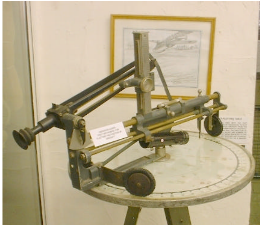
The Post Instrument that was used by the Observer Corps to establish the bearing, estimated height and position of aircraft during World War 2
