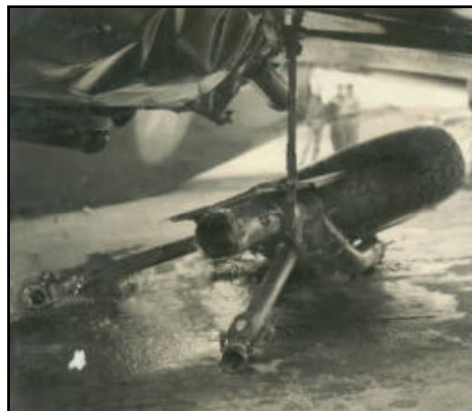
Sheared off undercarriage leg of B24D 41-23999
